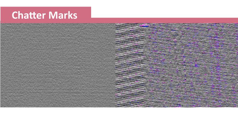
The left figure shows a roll without significant chatter marks. The right figure shows short wavelength chatter marks. In the left area there is a long wavelength chatter frequency below the short wavelength chatter mark.
