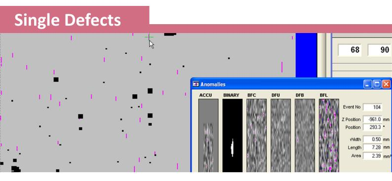
Different classes of Single Defects will be detected and classified through a flexible set of filters.
